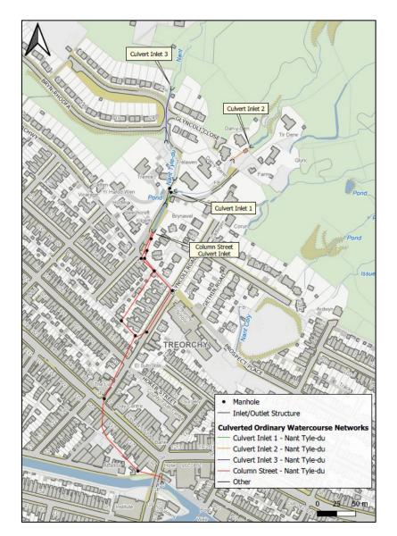
Figure 11: Surveyed culverted ordinary watercourse networks within the 'Nant Tyle-du' subcatchment
