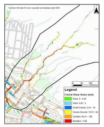
Figure 25: Critical shear street results in the Q100 flood event produced by JBA's hydraulic modelling
